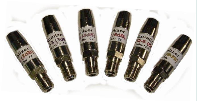
These RMS EQ equalizers have been designed for indoor/outdoor use. Each unit has been tested to 15psi (water test), The female contacts (F61) have a neoprene insert with a 360 degree contact which provides a high holding force. The male connector has an integrated "O Ring"
